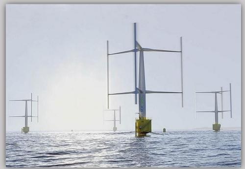
The Swedish company SeaTwirl is developing a vertical-axis floating wind turbine called S2x.
