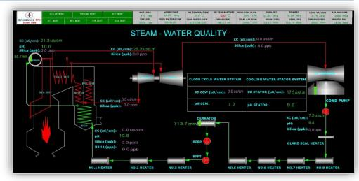
Vinh Tan thermal power plant has improved the installation, connection, and transmission of signals from the steam-water quality analysis system to the DCS system for online monitoring. providing timely alerts adjustments to maintain the quality of steam and water during operation, ensuring the plant operates safely, reliably, stably. This helps extend the lifespan of key equipment such as boilers and turbines.
