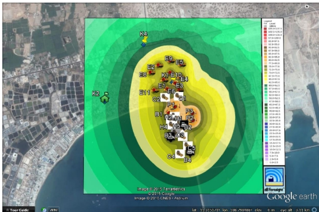
Figure 3.3. The noise contour map at the construction site of Vinh Tan 4 TPP and Vinh Tan 4 Ext TPP
